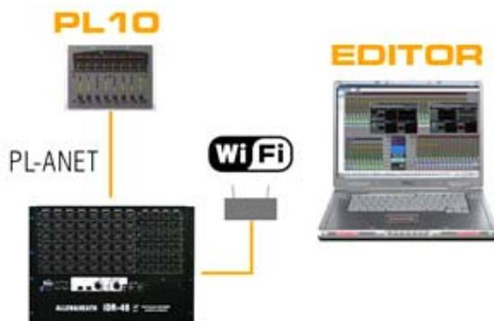
**Operating without a Surface** Leave your Surface at home and control iLive using just your laptop for compact or discreet mixing situations. You could add one or more PL Series controllers if you want to assign some physical control, for example important channels, DCAs or master levels.
